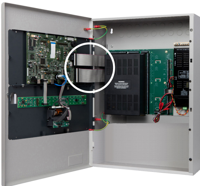
Figure 2-4 Removing Ribbon Cables
