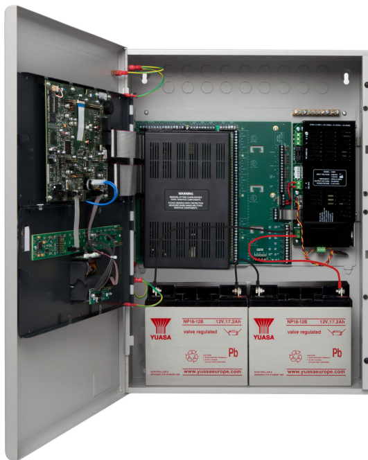
Figure 2-11 Connecting Standby-Batteries of the 5.25 Amp Power Supply
