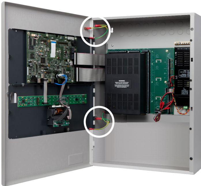
Figure 2-3 Removing Ground Connections
