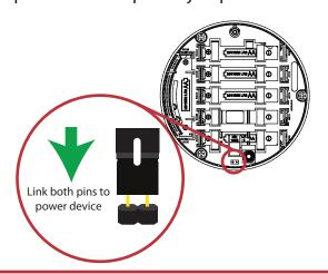
Combined sounder detectors are powered by changing the orientation of switch P as shown:
