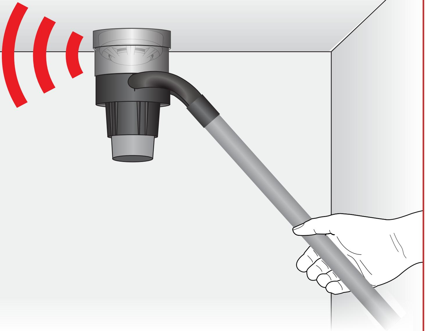
**Note:** loops can be entered into fast test for ease of testing. This allows the detectors on the selected loops to be triggered into an alarm condition quicker than normal. The led on the device will flash to indicate it is in this fast test mode. A time period of between 1 and 30 minutes is selectable which decrements and is then re-generated on a fire alarm event. The devices automatically come out of fast test mode when the timer expires or the fast test mode is exited.
