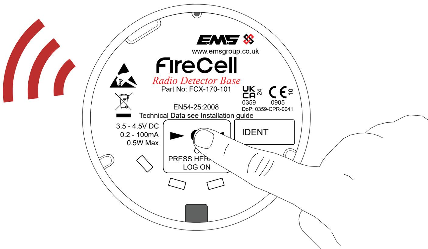
The wireless devices can be added to their relevant RCCs, either by pressing the device's log on buttons or by entering the device's unique ident number. If adding by ident, always make a note of the devices ident numbers and device type prior to installation and refer to the Programming Manual (MK98) for further details.
