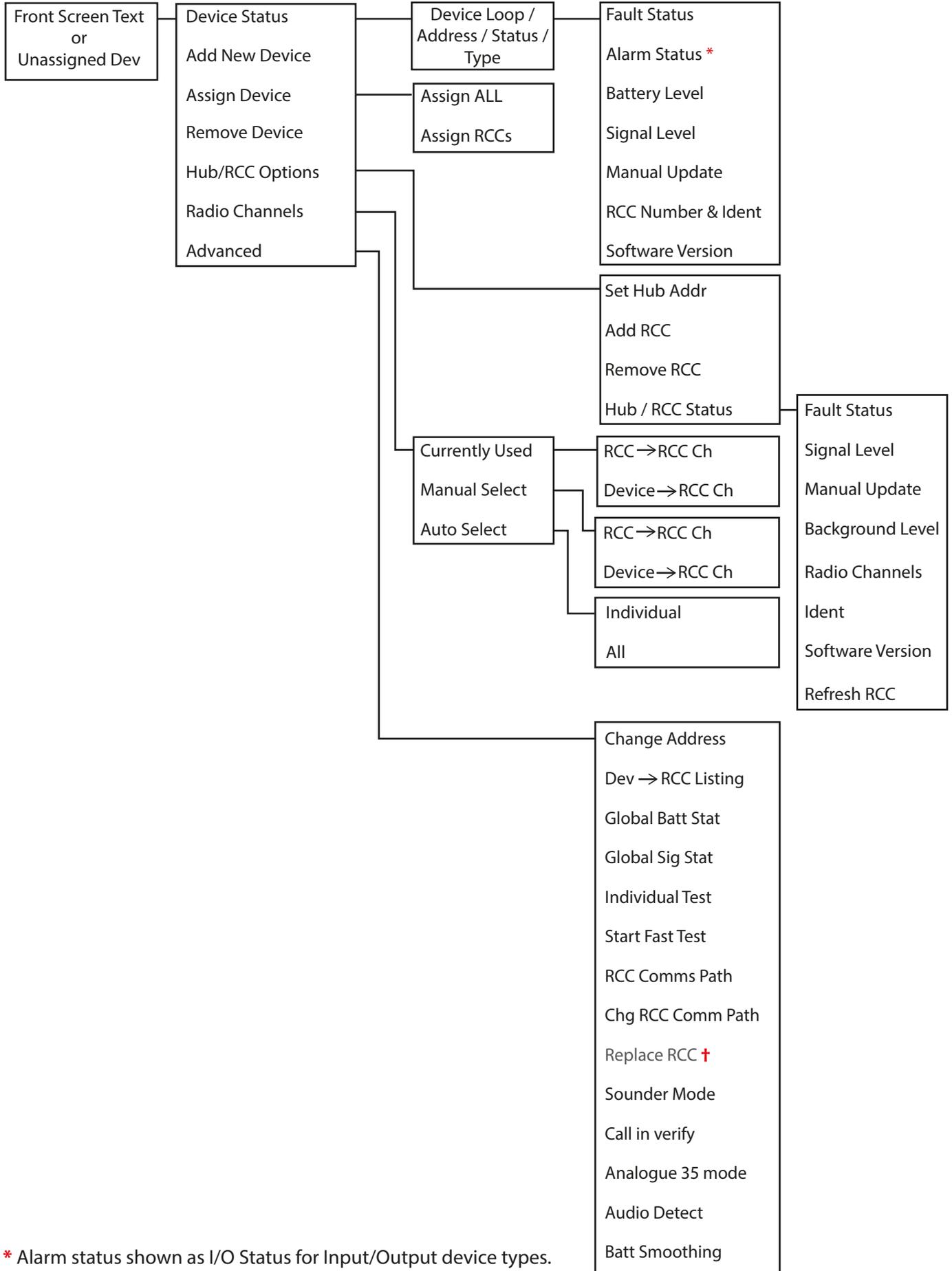
\* Alarm status shown as I/O Status for Input/Output device types.
