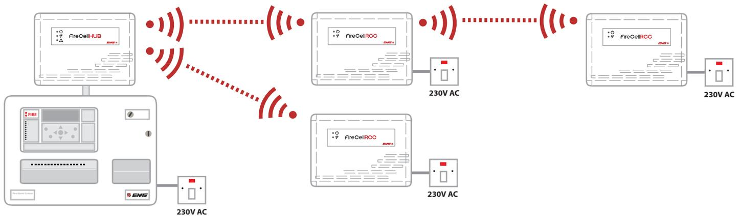
The RCCs (Radio Cluster Communicators) require installing in their proposed locations. Refer to the RCC Installation Guide (TSD053) for more information.
