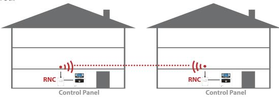
The recommended distance between metal objects from the aerial is 600 mm. The recommended distance to any other electrical equipment is 2 m.
