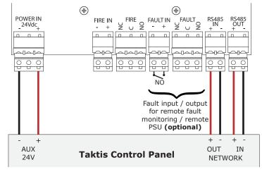
Please note: Care must be taken to ensure that connections are made correctly before applying power to the unit. Damage may occur if cables are incorrectly connected.
