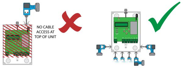
ALL CABLES TO BE ROUTED NEATLY AT THE BOTTOM OF THE BOX, AND NOT OVER THE PCB BOARD
