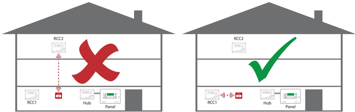
If not try moving the device to the correct / closest RCC. Details can be found within the FireCell Programming Manual (MK98).
