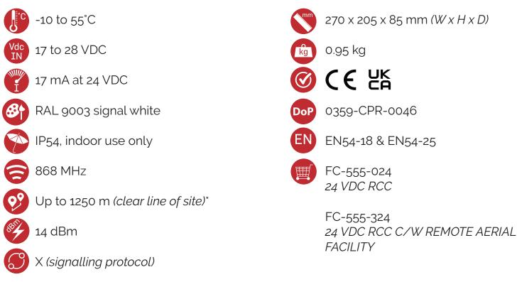
\*Line of sight refers to the maximum distance over which radio frequency signals can travel in a direct, unobstructed path between transmitter and receiver.
