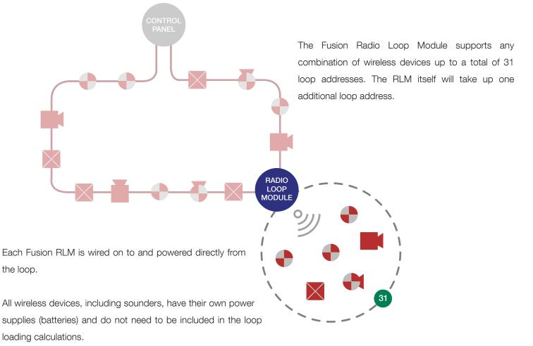
Each hard wired loop can support a maximum of five RLMs.
