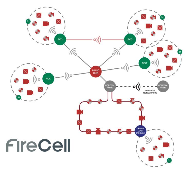
Based on EMS technology FireCell is fully scalable from standalone smaller single loop systems through to multi building networks.
