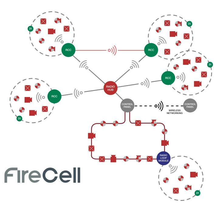
Based on EMS technology FireCell is fully scalable from standalone smaller single loop systems through to multi building networks.
