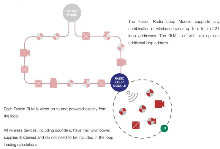
Each hard wired loop can support a maximum of five RLMs.
