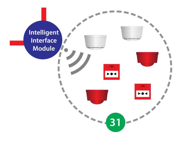
The intelligent interface module shall have LED indication of power status and fault indication.
