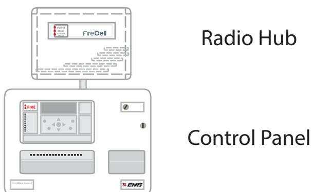
The Control Panel and the Radio Hub require installation into their proposed locations. (See the Radio Hub Installation Guide for more information).
