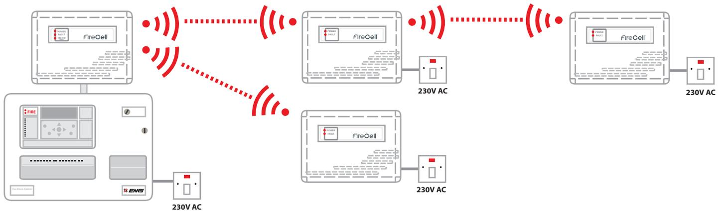
The Radio Cluster Communicators (RCCs) require installing in their proposed locations. Refer to the Radio Cluster Communicator Installation Guide (TSD053) for more information.
