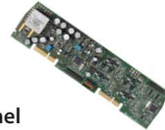
\*Note maximum 3x additional 2 loop cards can be added to the 2 loop panel
