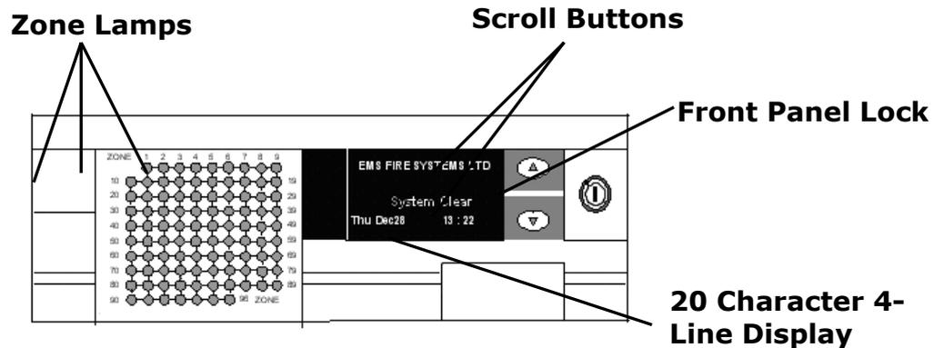
**Figure 1 - Zone Lamps and Display (96 Zone model shown)**
