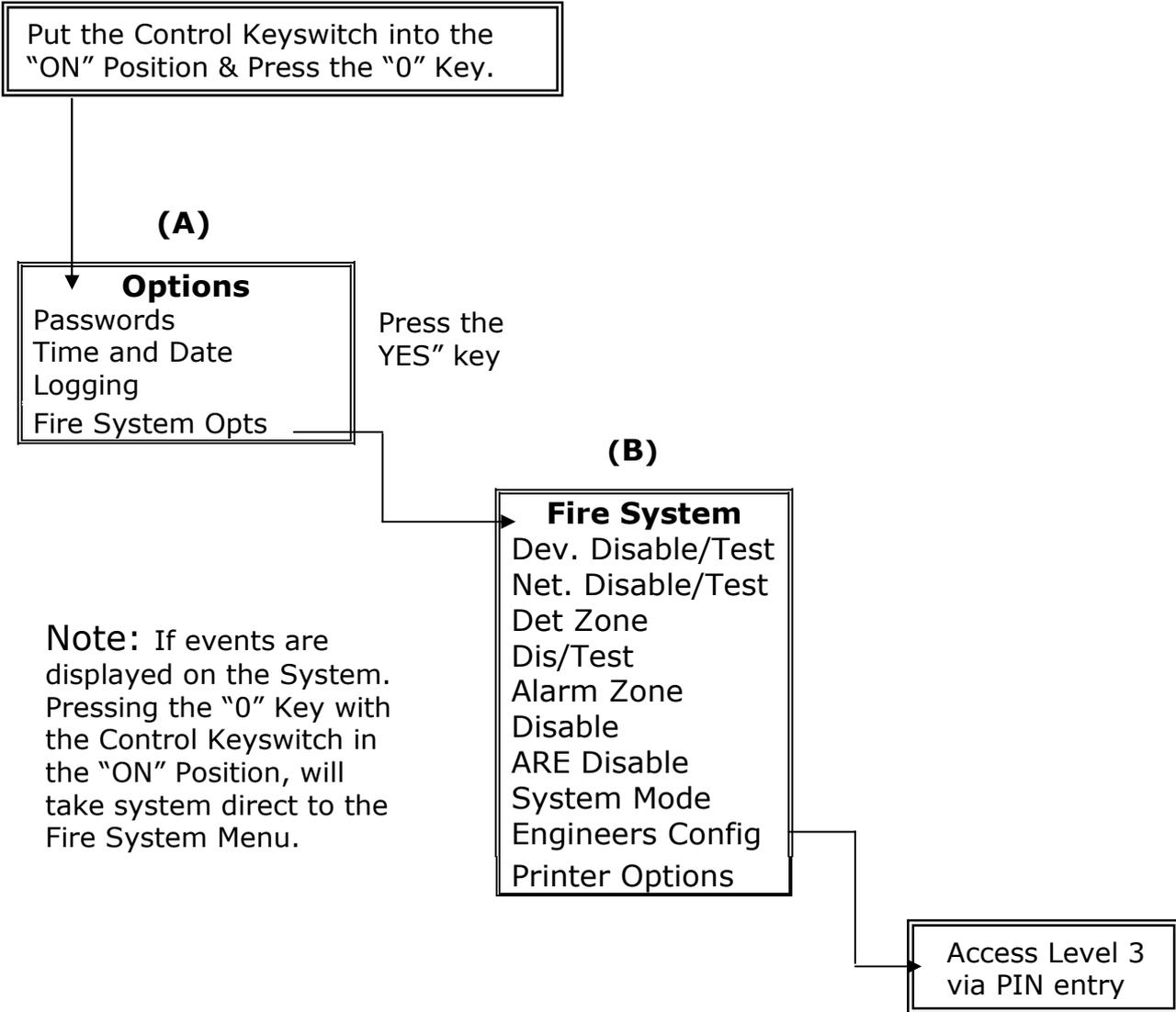
To scroll through the menus, use the "Δ" and "∇" scroll buttons. To enter a menu position the required option between the > and < cursors on the screen and press the "YES" key.
