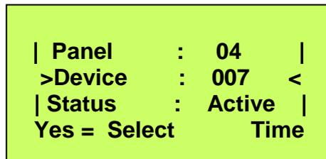
Press the ∇ key one time and the screen will change to highlight ">Status : Active<". Press "YES" key once to change the Status of the device to Active or Disabled as desired. Now press the ∇ key once and whilst highlighting ">Transmit Event<", press the "YES" key to transmit the event. The screen will state that the change has been made.
