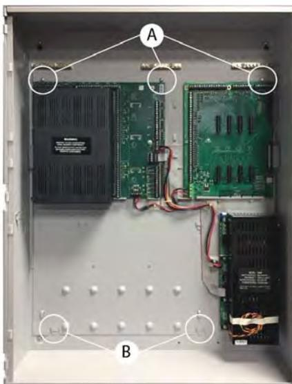
To remove the chassis from the Cabinet-Box:
