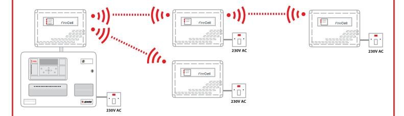
The Radio Cluster Communicators (RCCs) require installing in their proposed locations. Refer to the Radio Cluster Communicator Installation Guide (TSD053) for more information.
