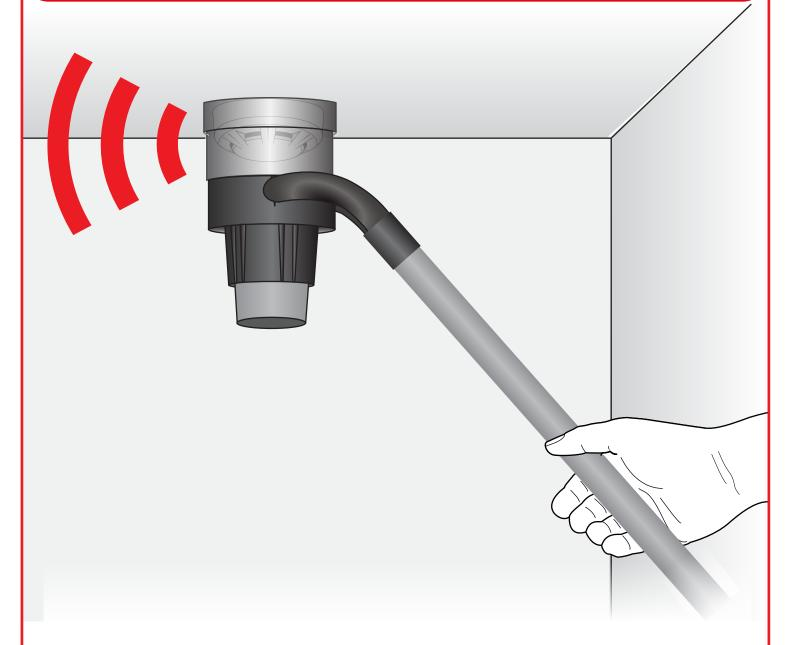
Note: loops can be entered into fast test for ease of testing. This allows the detectors on the selected loops to be triggered into an alarm condition quicker than normal. The led on the device will flash to indicate it is in this fast test mode. A time period of between 1 and 30 minutes is selectable which decrements and is then re-generated on a fire alarm event. The devices automatically come out of fast test mode when the timer expires or the fast test mode is exited.
