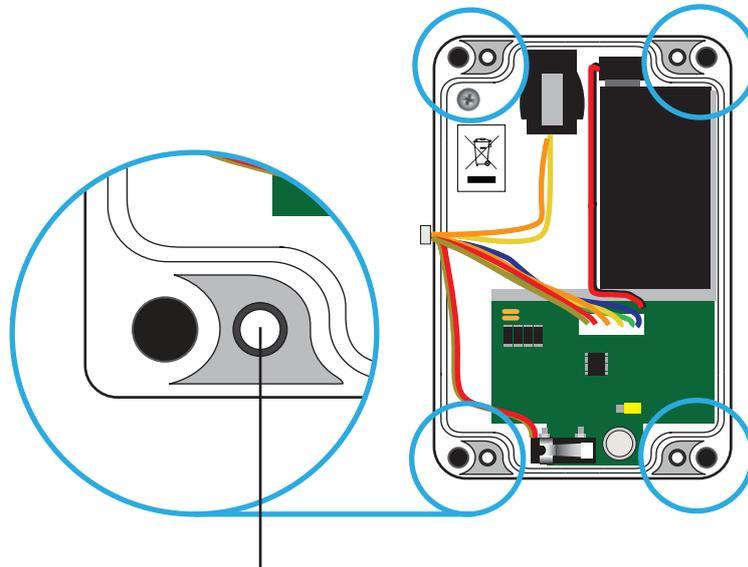
Fixing position location within cavity
