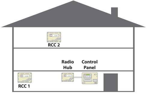
The recommended distance between metal objects from the aerial is 600mm. The recommended distance to any other electrical equipment is 2 metres.
