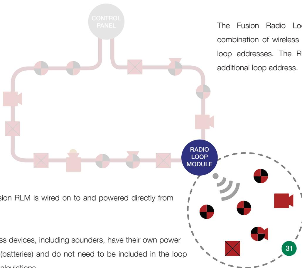
The Fusion Radio Loop Module supports any combination of wireless devices up to a total of 31 loop addresses. The RLM itself will take up one additional loop address.
