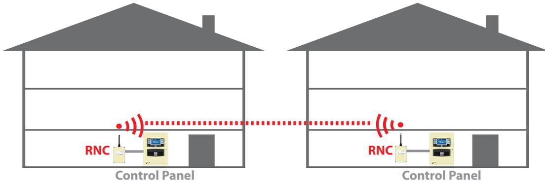
The recommended distance between metal objects from the aerial is 600mm. The recommended distance to any other electrical equipment is 2m.
