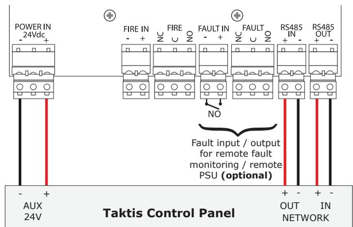
**Please Note: Care must be taken to ensure that connections are made correctly before applying power to the unit. Damage may occur if cables are incorrectly connected.**
