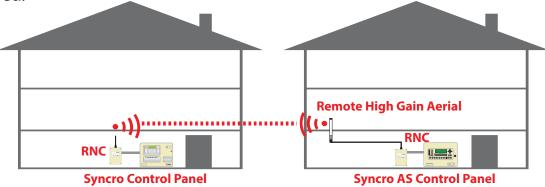
When connecting an RNC to a Syncro 2 or 4 loop Panel, the recommended distance between metal objects from the aerial is 600mm. The recommended distance to any other electrical equipment is 2m.
