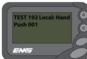
Note: The test value shown is not able to identify which receiver has actually received the signal. If this method of testing is required, refer to Page 13 .
