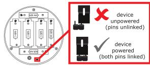
Once powered, reassemble the device.
